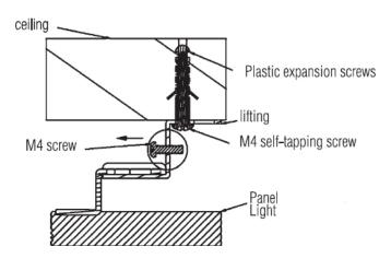
E: Loosen the M4 screws which are in the Step B to the location as illustration showed. Attention: This is the combination darwing between a single lifting
