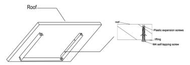
B: Fix the AL frame to the roof with M4 screws on both sides of drilling hole as illustration shown.
