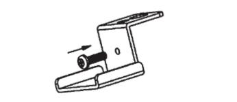
B: Nail M4 screws into lifting devices in the direction as the arrow shown. Attention: The screws should be nailed to the bottom.
