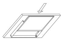
C: Placing the panel light in the slot of AL frame along the level line as required. Please ensure the panel light is recessed in a stable and even position.
