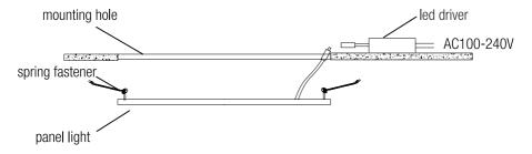
C. Pls connect the power input line with the electric supply, and power output line with the panel light.
