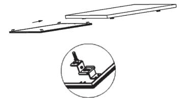
C: Put the LED panel on the lifting devices in the direction as illustration showed.
