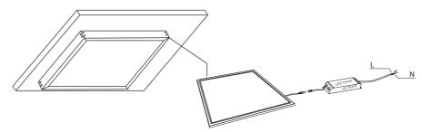
D: Connect the power driver to the panel hidden in lamp's back. Check the safety contacts. Tighten the missing constructure with screws to finish the installation.
