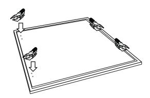
2. Make a mounting hole suitable for the luminaire
